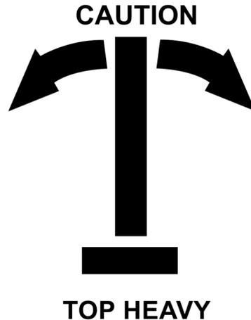
Top-heavy articles are those having a center of gravity higher than  $\frac{1}{2}$  their standing height and having a height of two times or greater of the shorter base dimensions, as packaged.
